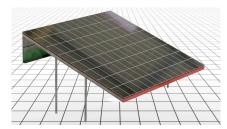
Structure fully covered with Solar 260-watt PV Panels: 204 kW Total.
